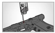
Easily remove all pins to disassemble your Glock to clean, modify or maintain
