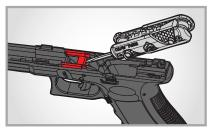
Remove & install internal components like the slide lock spring & locking block with small flathead driver
